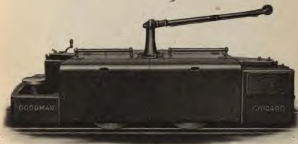
A "Safety-First" Locomotive, with Guarded Wheels
